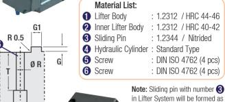
If J>0: On mould surface which system will be mounted: A discharge will be performed in dimensions of "D+2mm x (A+P)+3mm x J+1mm"
